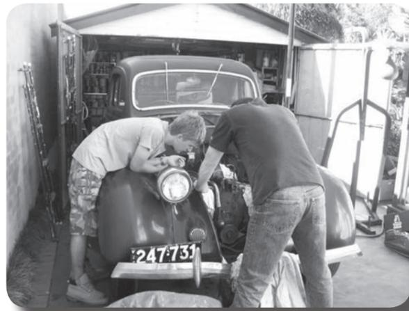
ABOVE: Preparing the engine for removal.
