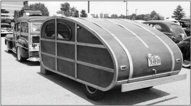
1947 Ford Woody Wagon towing a 'Fleet' Cabin-Car teardrop trailer. N.B. Rearward position of the single axle!
